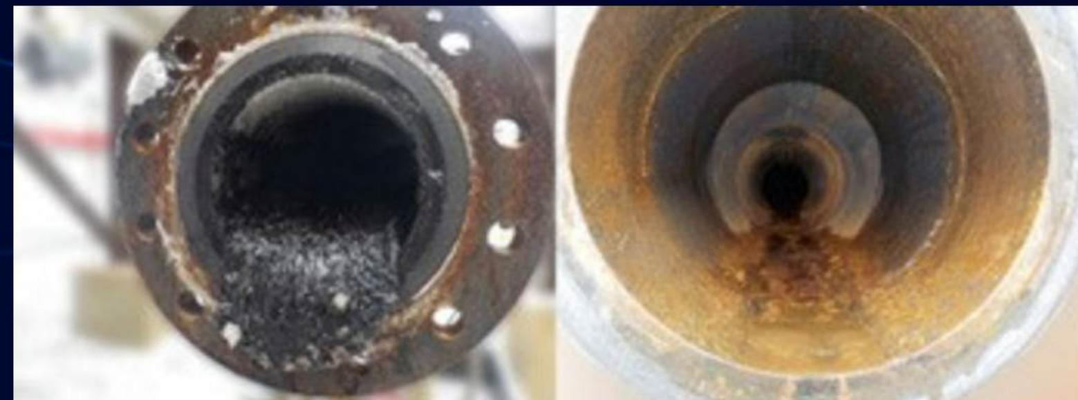
Common methods to combat paraffin deposition like mechanical cleaning (slick line tools and pigging methods) electric heating, ultrasonic and microbiological treatments (for breaking down paraffin deposits) , paraffin Inhibitors (chemical solutions to prevent wax formation) - remains with limited efficiency.
